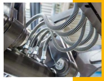
The skid steer loaders place high demands on the hydraulic hose lines. The bending radii were successfully optimised without obstructing the flow in the hydraulic circuit.
