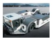
AN AIRCRAFT TOWING TRACTOR WITHOUT A TOWBAR FROM TREPEL
