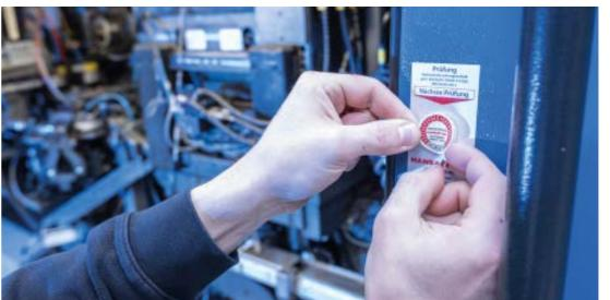
After the maintenance work has been successfully carried out, the next period for preventive maintenance is determined and documented with a sticker directly on the machine. This prevents any unscheduled downtime.
