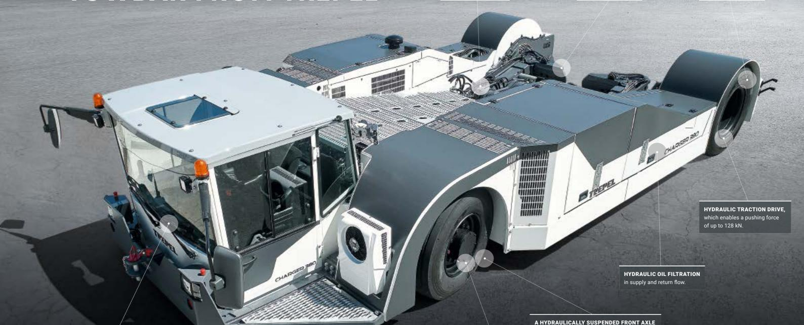
SUSPENSION LIFT CAB hydraulically height adjustable from 1,650 mm to 1,960 mm.
