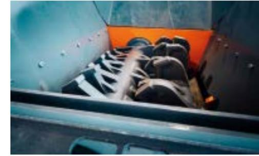
◀ The asynchronously driven shafts crush materials of all kinds. The quick-change cassette developed by Arjes allows tools to be changed within a short time.
