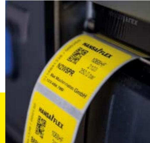
The new hose label displays all relevant data such as the manufacturing date of the hose line and the X-CODE. Customer-specific information can also be printed.
