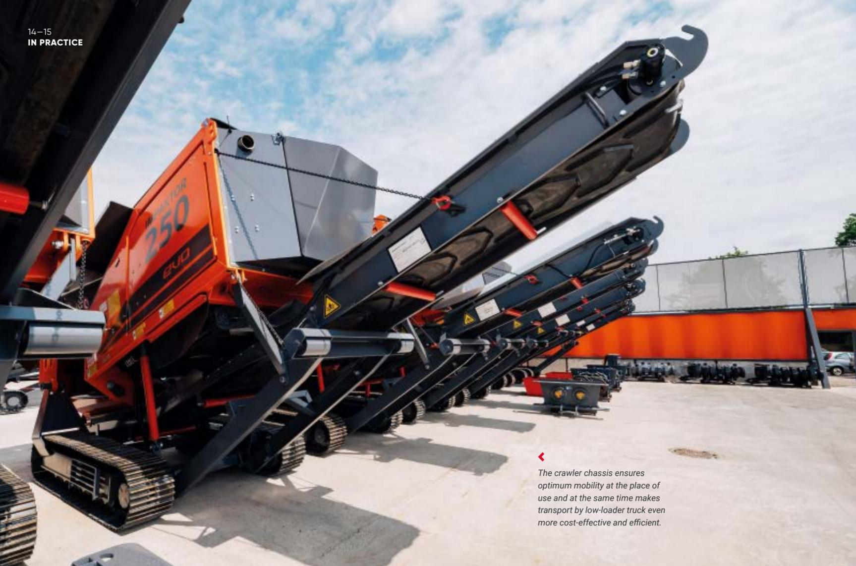
◀ The crawler chassis ensures optimum mobility at the place of use and at the same time makes transport by low-loader truck even more cost-effective and efficient.
