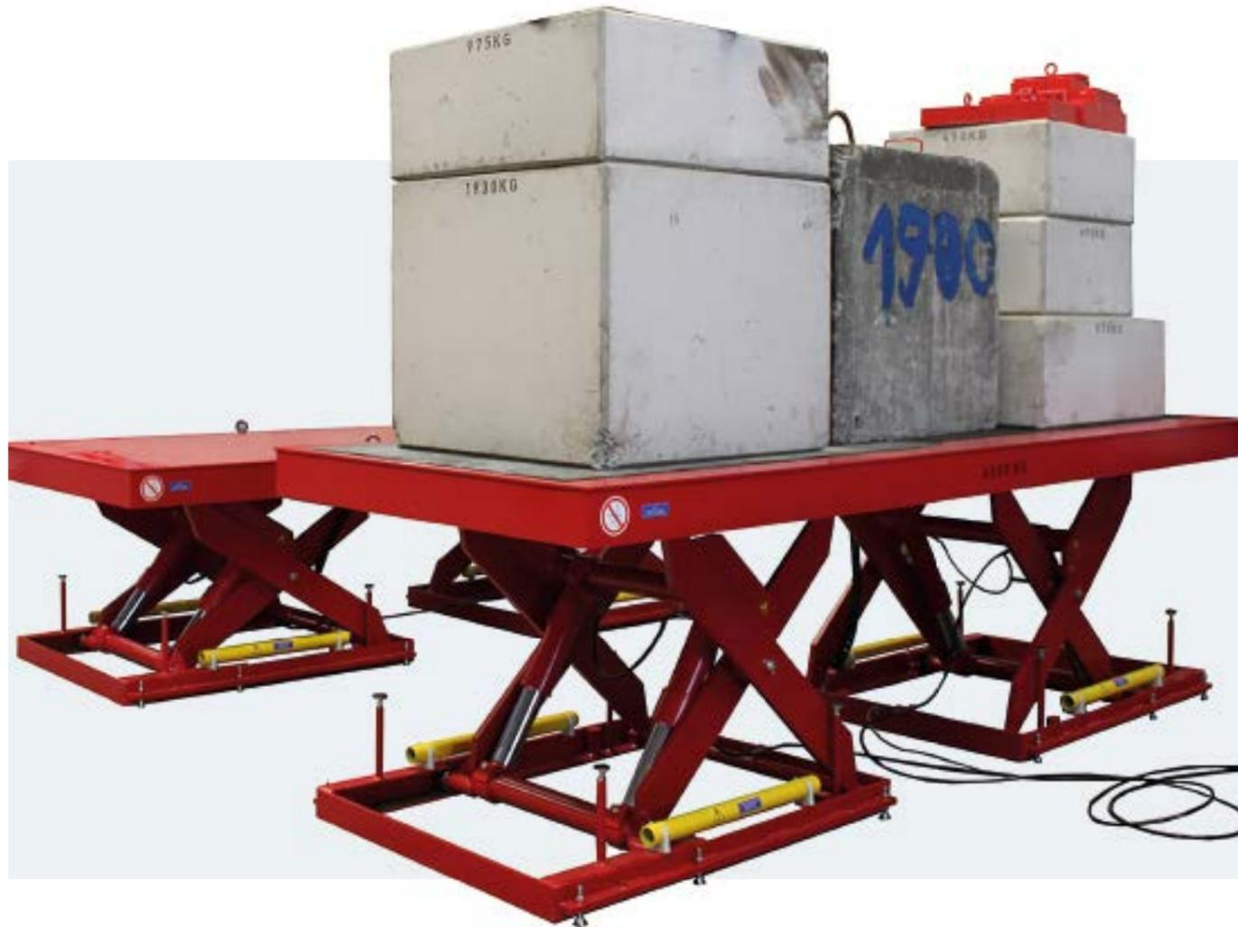
Sample application: scissors lift table from Janzen-Lifttechnik. The lowering brake valve is already integrated and pre-set in the cylinder connection (on the piston side)!
