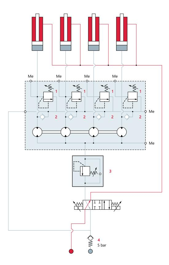
(1) Phase correction valve in the gear flow divider
